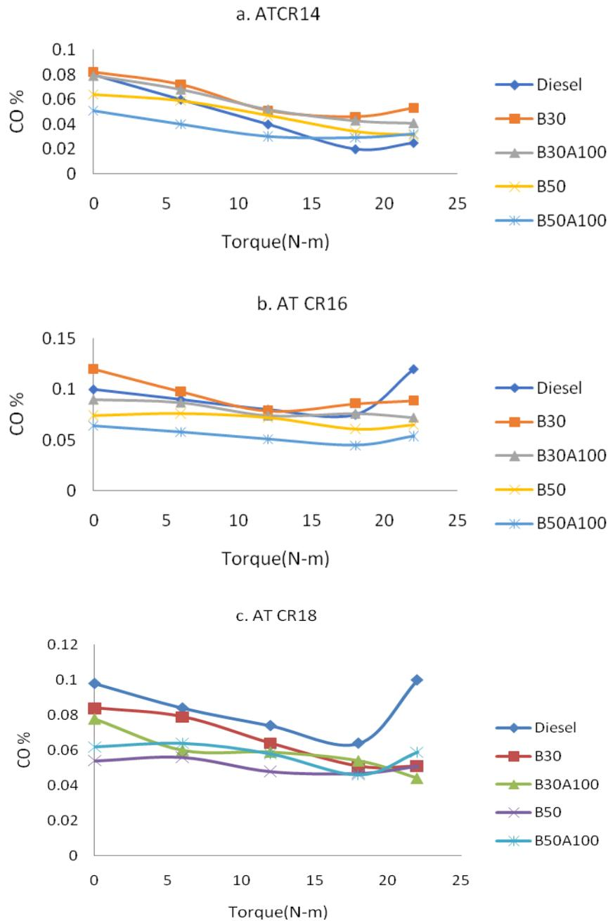
**Figure 3: Variation of carbon monoxide with torque at different compression ratios**
