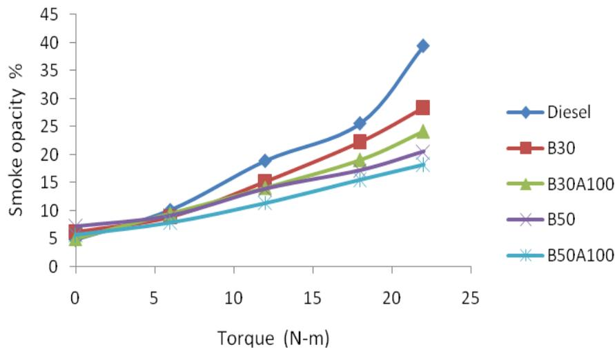
Figure 6: Variation of Smoke Opacity with torque
