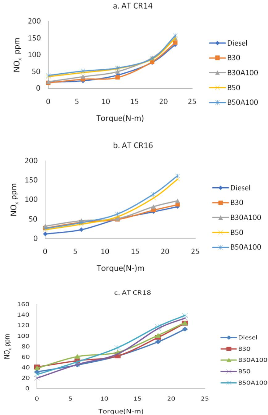
**Figure 5: Variation of Nitrogen oxides emission with torque at different Compression ratios**
